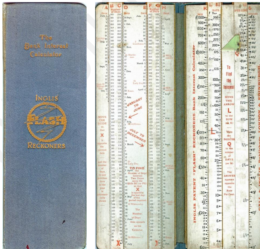
Fig. 24: Inglis' 243x80x6mm Flash Reckoner - Bank Interest Calculator
