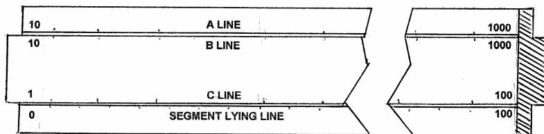
*Figure 5. The Head Rod: scheme of lines (face side above, reverse side below)*
