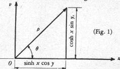
Methods of changing to the polar form  $\rho/\theta$  by use of the slide rule will now be explained. First, it should be noted that the real number y may be expressed in either radians or angular degrees. Since the graduations on the S and T scales are in terms of degrees, this measure is more convenient. A value of y given in radian measure should therefore first be converted to angular degrees.
