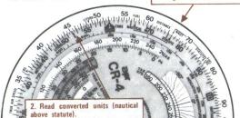
Note that by aligning nautical and statute mile indexes, any number of units may be converted progressively without resetting the computer.
