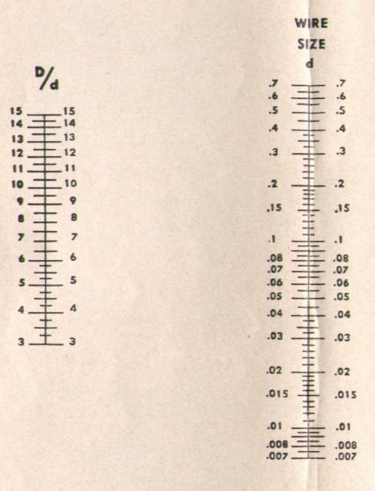
To use the chart, calculate the ratio D/d. Then lay a straight-edge (transparent celluloid is best) so that it connects the value of D/d on the left-hand scale with the value of the wire size on the middle scale. The amount of initial tension is then read on the right-hand scale, in pounds of pull required to bring the spring to the point where the coils begin to separate.
