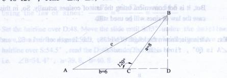
Draw a vertical line from B and intersect with the extension line of AC at D. Then,
