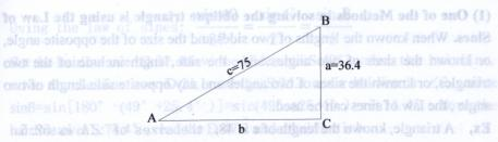
read the S:29 under hairline is the  $\angle A$  and its complementary angle S:61 ° is  $\angle B$ . Move the hairline over S:61°, read the D:65.6 under hairline is the b.
