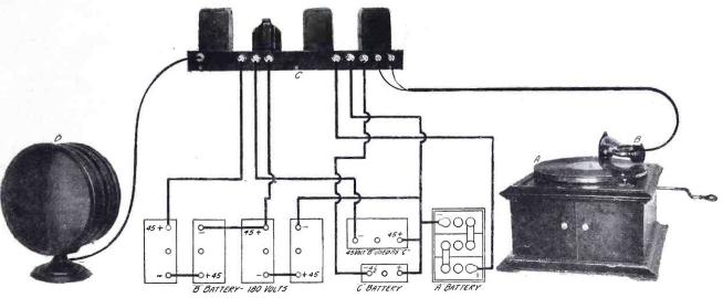
ANOTHER MATCHED COMBINATION THAT EMPLOYS DOUBLE-IMPEDANCE COUPLING AND TRANSFORMER COUPLING
