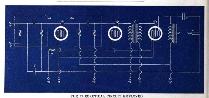
FIGURE 3: Here is shown the schematic diagram of the amplifier. The units indicated by dotted lines, A and B, are complete resistance-coupler units that couple the two tubes, G1 and G2. These are followed by a high quality transformer, C, and a power tube, G3. The ortput circuit contains a filter that improves quality, at the same time protecting the loud-speaker from heavy DC currents.
