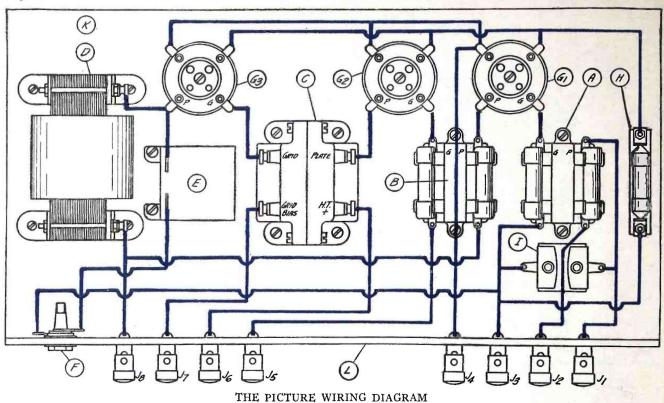
FIGURE 2: This drawing shows exactly how to hook up the various instruments in their respective electrical places in the circuit. The heavy blue lines indicate the wiring, while the black lines indicate the outline of the instruments themselves.
