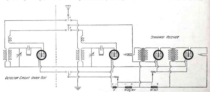
A SIMPLE RECEIVER AND TEST SET-UP
