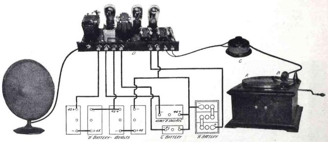
A MATCHED COMBINATION THAT USES RESISTANCE COUPLING AND TRANSFORMER COUPLING
