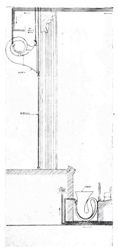
AN INSTALLATION IN A THEATER When the exponential horns of a public address system are installed in a theater, one or more horns are placed in the orchestra pit and another set is hung behind the curtain, at the top of the stage.
