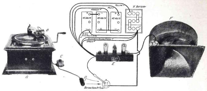
HOW THE NEW UNITS ARE CONNECTED TO A STANDARD PHONOGRAPH
