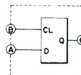
Fig. 2b — Synchronizer circuit with leading and trailing edges synchronized.
