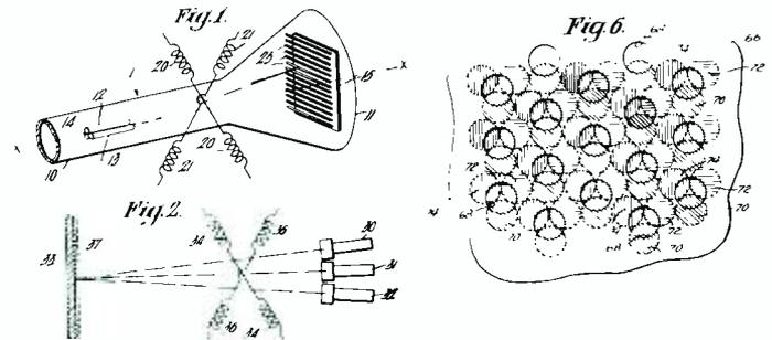
Selected figures showing three beams deflected by a single deflection yoke and the relative arrangement of mask apertures and phosphor dots that produces a nested phosphor-dot screen.
