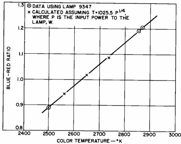
Fig. 5 — Blue-red ratio as a function of the lamp (NBS 9347) color temperature. The circled points are the blue-red value for NBS calibration temperatures. The crossed points were measured blue-red for temperature calculated from the input power to the lamp, assuming that  $T = 102.5 P^{1/4}$ , where  $P$  is the input power to the lamp, and the constant was selected for agreement with the NBS data at 2856 K.
