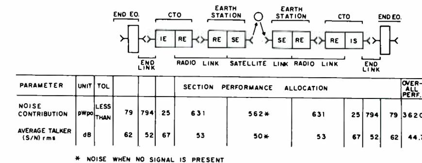
Fig. 11 — Transmission performance objectives for a private line voice channel (SCPC).
