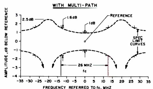
Fig. 5c — Transponder small-signal amplitude response specification limits.
