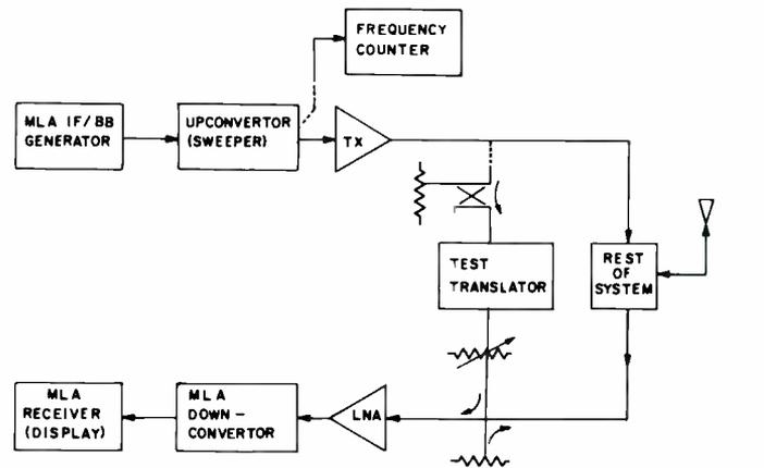
Fig. 4 — Amplitude response and group delay test setup.
