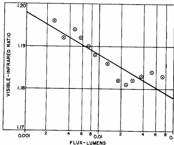
Fig. 6 — Ratio of the silicon photocell current for the visible (HA-11 filter) to the photocurrent for the infrared (a pair of CS 7-56 filters) as a function of the flux in lumens. Light source was a tungsten standard lamp. Note that the ratio decreases about 1% per decade as a result of the supralinearity characteristic of the silicon cell in the near infrared.
