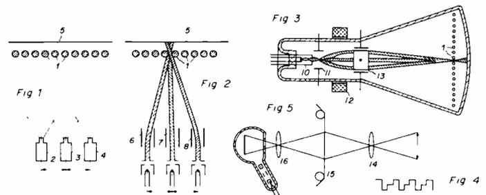
Figures show shadow-mask color-tube principles in a grill-type tube.
