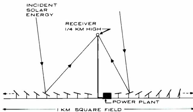
Fig. 4 — Schematic diagram of a central-receiver type of solar thermal electric converter. A field of sun-tracking mirrors approximately 1 km<sup>2</sup> is capable of generating nearly 100 MWe (electrical) during peak sunlight hours.
