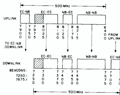
Fig. 1 — DSCS phase II satellite frequency translation plan.
