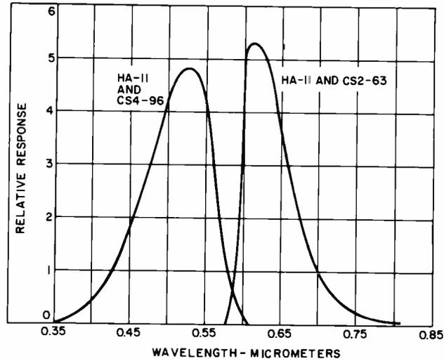
Fig. 4 — The relative spectral output of the silicon cell excited by tungsten-lamp radiation through the blue and through the red filters.
