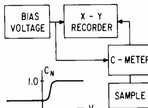
Fig. 1 — Conventional high frequency C-V measurement.
