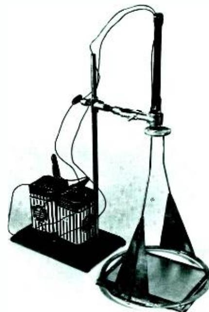
Fig. 1 — Lighthouse used in printing the first experimental shadow-mask color tube. A photosensitive film is located in the phosphor-screen plane. It is exposed from a point source in the lighthouse and through the shadow mask to locate the desired phosphor dot positions.
