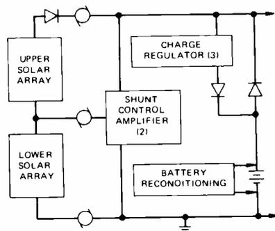
Fig. 3 — Power supply subsystem.
