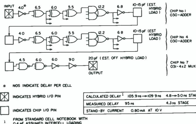
Fig. 7 — Adder hybrid measured performance.
