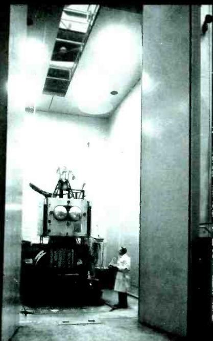
Dick Hartenbaum, AED engineer is checking the preparation of the satellite for exposure to high level acoustic energy (i.e. noise) simulating the launch environment.
