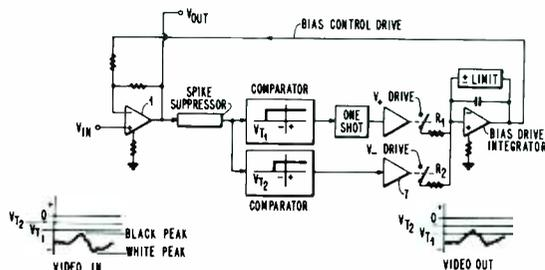
Fig. 1 — Circuit used to establish black level automatically.
