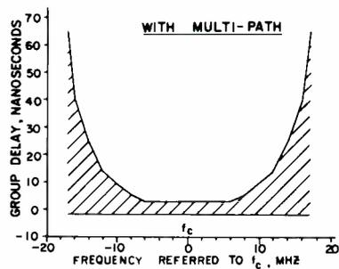
Fig. 5b — Transponder small-signal group delay response specification limits.
