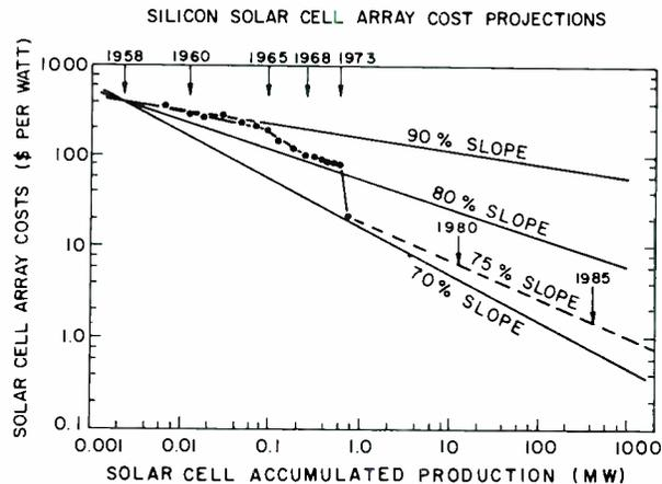
Fig. 2 — History (solid) and projection (dashed) of the cost of silicon solar-cell arrays. The association of fixed production levels with the years 1980 and 1985 are estimates that are dependent on the extent of the commitment made to this technology (adapted from Ref. 7, p. VII-C-64).
