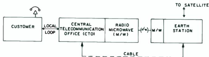
Fig. 1 — Signal flow from customer office to earth station.
