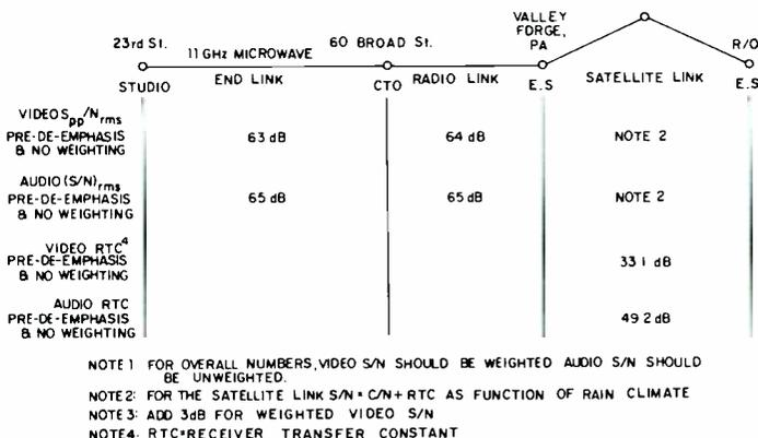
Fig. 7 — CATV television service. Hypothetical reference circuit for video and audio signal to noise ratio.
