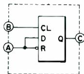
Fig. 2a — Synchronizer circuit with leading edge synchronized.
