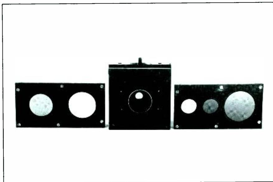
**Fig. 2 — Silicon photocell housing and the sliders with color filters used in the tungsten lamp calibration. From the left, the filters shown are: green (photopic match), infrared absorbing, open aperture, red, and blue. The small light circle which may be observed in the center of the housing is the front surface of the silicon cell shown through a 1/2 in. aperture.**
