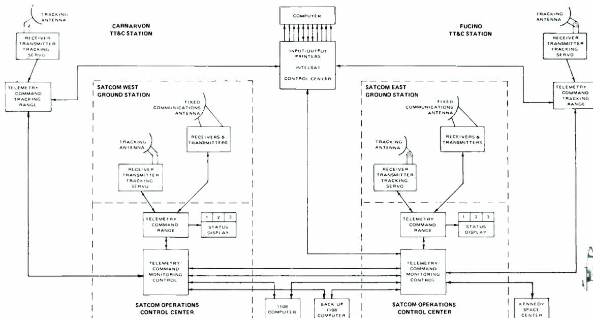
Fig. 8 — RCA Satcom mission operations complex.
