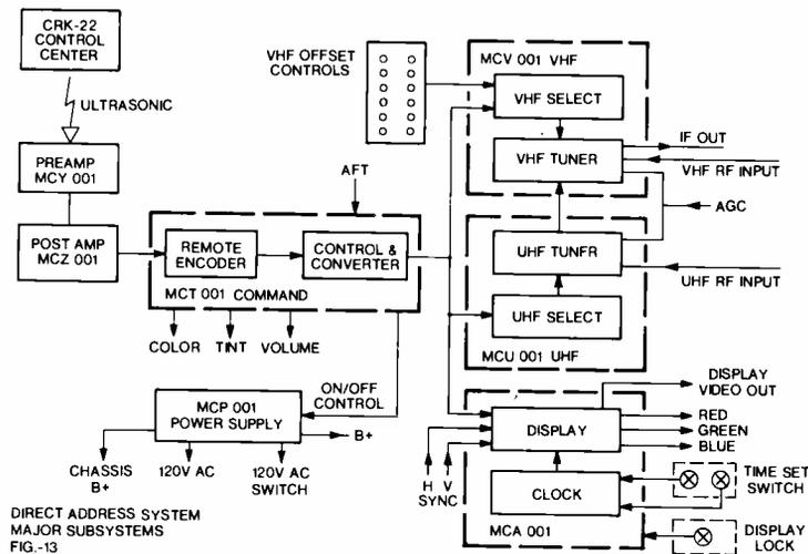
Fig. 13 — Direct address system major subsystems.
