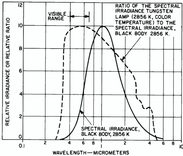
Fig. 1 — Relative spectral irradiance from a black body at 2856 K and the ratio of the spectral irradiance from a tungsten lamp operated at 2856-K color temperature to the spectral irradiance from a black body at 2856 K. Note that in the visible range, 0.4 to 0.7 micrometers, the spectral irradiance from the tungsten lamp closely matches that of a black body.
