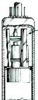
Fig. 1 — Electron gun structure.
