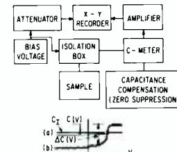
Fig. 2 — Modified high-frequency C-V measurement.
