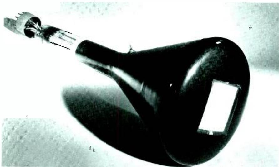
Fig. 2 — Experimental shadow-mask tube used to display color pictures on this type of color tube for the first time.
