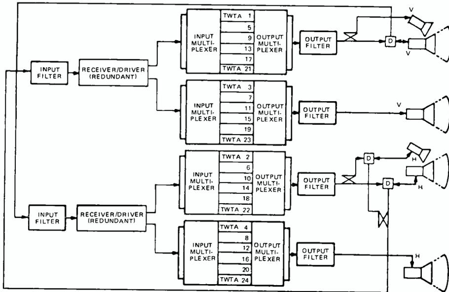
Fig. 1 — Transponder and antenna assembly block diagram.
