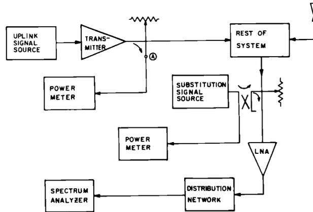
Fig. 1 — EIRP (effective isotropic radiated power) and flux density test setup.
