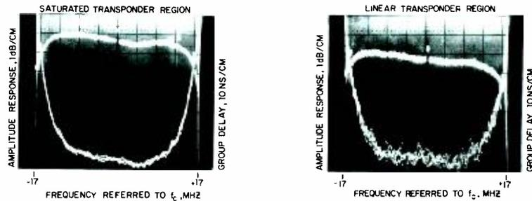
Fig. 5a — Transponder amplitude and group delay responses.
