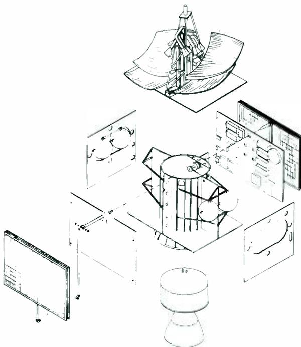
Fig. 5 — Exploded view of spacecraft.
