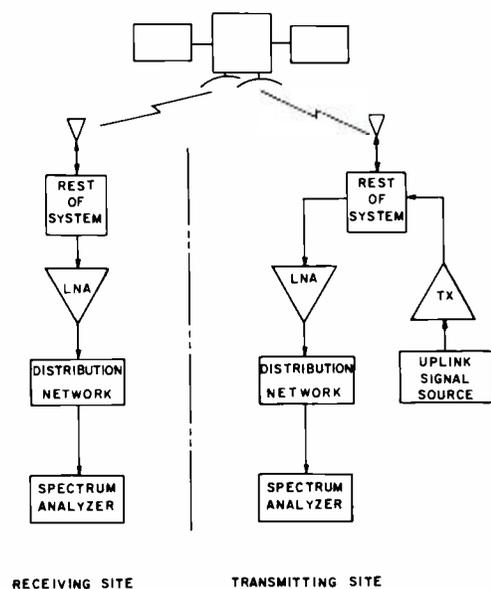
Fig. 6 — Cross polarization isolation test setup.
