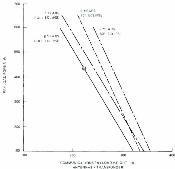
Fig. 10 — Spacecraft payload capacity.
