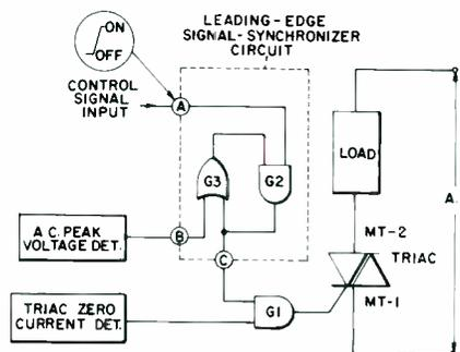
Fig. 1 — AC power control system.
