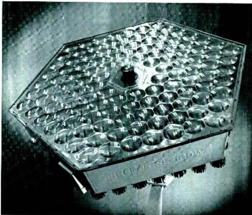
Fig. 3 — One version of a photovoltaic array using concentrated sunlight. The front cover is a molded plastic panel of lenses, each focusing its light onto a cell 1000 times smaller. The dark protrusions at the back are ordinary heat diffusers that limit cell heating to 20°C. At front center is a set of sun sensors that control the direction of the array (Courtesy L. Napoli, RCA Laboratories).
