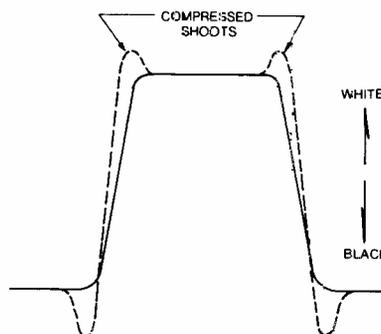
Fig. 9 — Transversal filter peaking.
