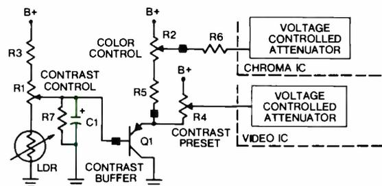
Fig. 3 — Contrast circuit and light-dependent-resistor.
