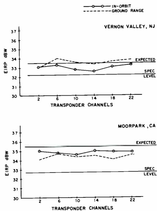
Fig. 2 — Typical EIRP performance (transponders 2, 6, 10, 14, 18, 22).
