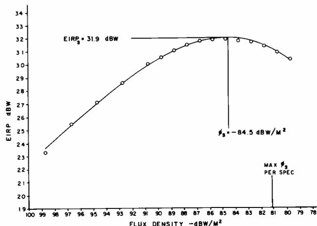
Fig. 3 — RF-power transfer curve (transponder 2 from Vernon Valley, N.J.)
