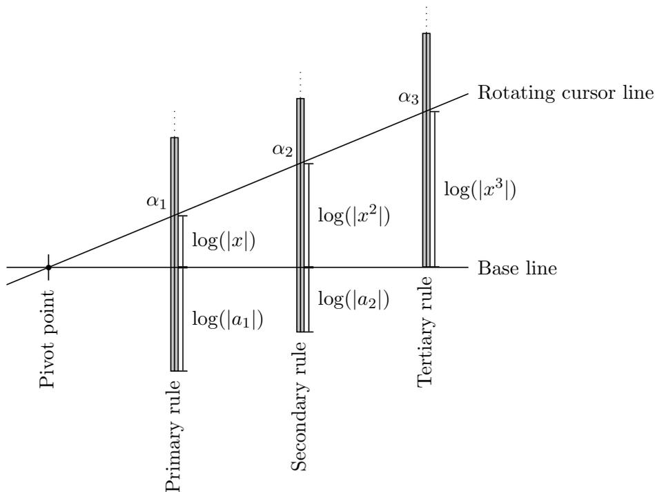
Figure 1: The principle of Newton's polynomial solver
