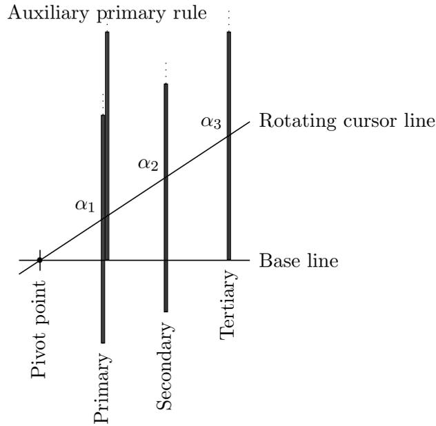
Figure 2: Reading  $x$  directly with an auxiliary primary rule.
