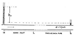
96. Any other value of  $h_v$  could have been used in The Specifications without changing any of the Basic Ratios. The Force always equals The Resistance; therefore, The Ratio  $h_v \div f_v$  is always maintained.
