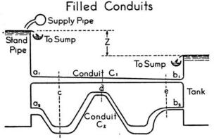
1. When through any filled Conduit a Fixed Volume (Bbls. per day, Liters per minute, etc.) of any Liquid is regularly passing an up-stream point (a), passing on through the system and passing a down-stream point (b), Then the same Fixed Volume passes each point along the route in the same length of time. The Liquid, the material and shape of the Conduit or the roughness of its surface, do not change the condition of Steady Flow.
