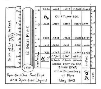
Any difference in head,  $h_v$ , divided by its corresponding length, L, is the head required for one foot in length of the Pipe. The  $h_v$  of the Specifications is for 10,000 feet of 1 ft. Pipe. This is a measurable quantity.
