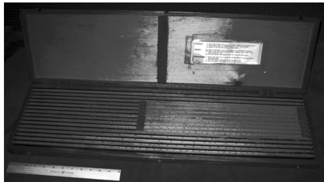
Figure 9. Hannington’s gridiron slide rule—courtesy of Bob DeCesaris [14]
