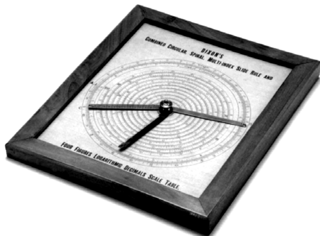
Figure 4. Dixon's Combined Circular, Spiral, Multi-Index Slide Rule, ca.1882—Science Museum/Science & Society Picture Library, London [59]
