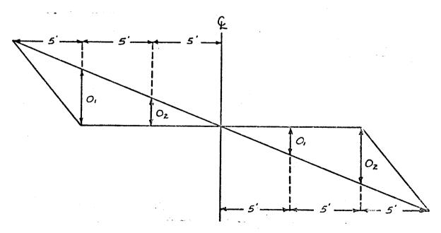
Area Triangle (cut) =  $(0_1 + 0_2) \times 5$ Area Triangle (fill) =  $(0_1 + 0_2) \times 5$  The "Avol Rule" is a commercially available plastic scale that automatically totals the vertical distance and multiplies by the spacing.
