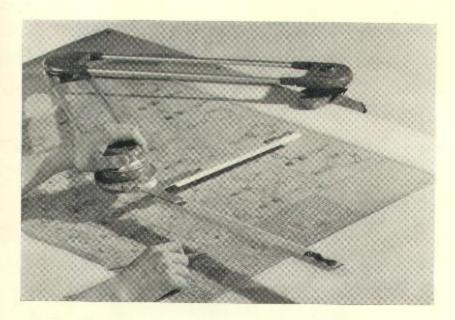
The big idea is, it permits you to move a rule all over a drafting board and the rule stays parallel to its original position. The best model works on the principle of enclosed drums and steel bands. The accuracy depends on the precision of the radii of the drums, if I am not too stuffy.
