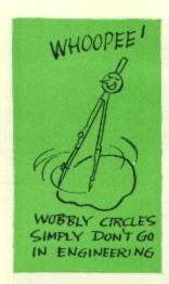
moving parts. The joints mean a lot (as whose joints don't?). The accuracy of the instruments depends on them. If the joints of a compass wobble, you'll draw a wobbly circle. That is, if the joints of a compass don't move in the same plane, the points of the instrument won't meet exactly. You'll get eccentric circles, which don't go in engineering.
