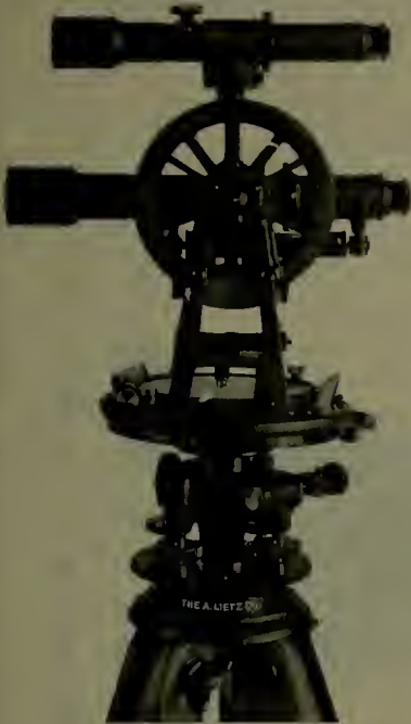
Showing Secondary Telescope in position on top for measuring horizontal angles.
