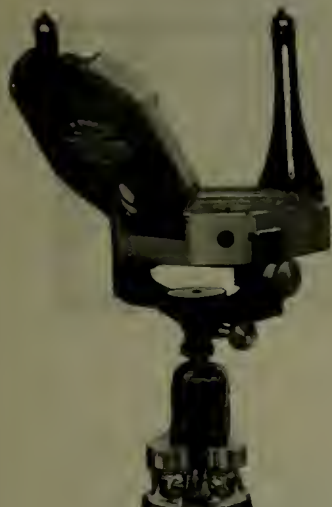
Showing Brunton Transit on Ball and Socket Tripod Head No. 185C.
