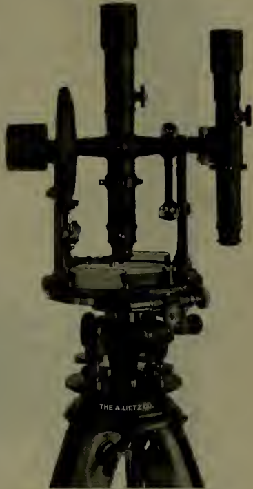
Showing Secondary Telescope in position on the side for measuring vertical angles.
